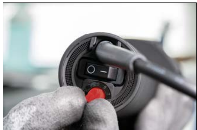
Adjusting H6100 operation temperature.
