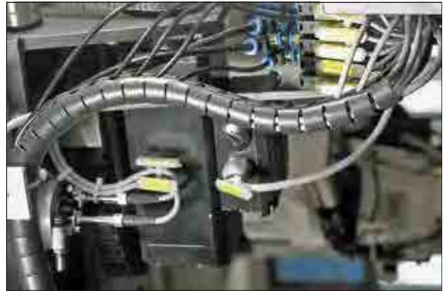
Cables can be branched off at any point for better, more flexible protection.
